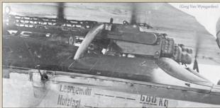
Cockpit coaming and high mounted LMG 08/15 'Spandau' detail from Julius Bender's Jasta 4 Fokker D.VII F seen on page 6. Note the padding.
