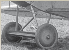
^ Undercarriage detail from Daimler-Mercedes powered Fokker built D.VII 379/18 showing early production painted wheel covers with Fokker style inner tube valve access panel.
