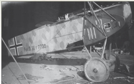
The fuselage of late production Fokker D.VII F 7732/18 is covered in 4 colour lozenge material. The wheel cover and (unusually) the triangular access hatch (116) also appear to have been covered with lozenge fabric.
