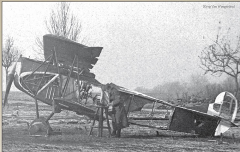
This unidentified captured Fokker D.VII F has been enthusiastically ransacked by American souvenir hunters. Note the unpainted area where the side cowl overlaps the underlying cowlings, late style rear cowling (115) and the single carburetor (121) of the BMW IIIa engine. The cut out in the nose cowling above the propeller is similar to that seen on some Jasta 10 aircraft.
