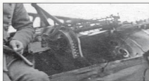
Cockpit coaming and high mounted LMG 08/15 'Spandau' detail from Erich Just's Fokker D.VII F 460/18
