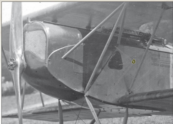
Nose detail from early production Fokker D.VII 379/18 as seen on page 17 showing smooth cowl (15) and full length fuselage fabric (12). The bottom of the undercowl (A29) appears to have been painted light blue while the edges remain dark green(?) like the nose cowls.
