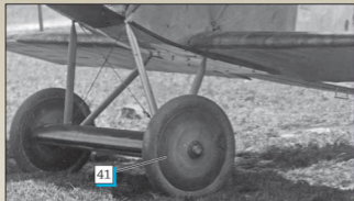
Undercarriage detail from D.VII 379/18 showing painted wheel covers with Fokker style inner tube valve access panel and 'Innen' stencil 41 which is only faintly visible.
