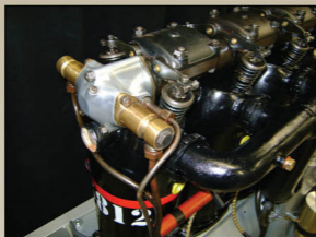
Detail of the horizontal air pump associated with the 200hp engine.
