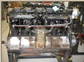
Left hand side of the engine, the red-brown pipe carries the plug leads from the magnetos to the spark plugs.
