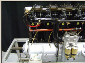
Water jacketed intake manifold and carburetor detail. A mount for the generator (P43) can be seen at right but the actual generator was very rarely installed in fighter aircraft unless used to power an electrically heated flight suit or wireless transmitter.
