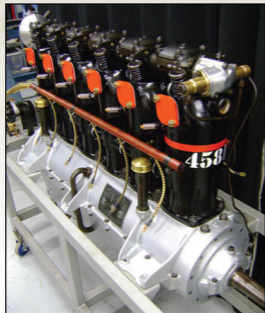
Unlike earlier versions of the Daimler-Mercedes D.III and D.IIIa, the engine numbers appear to have been regularly applied to D.IIIaü engines installed in the Fokker D.VII and we have supplied decals [32] & [33] for you to choose from. The red bands [35] & [36] are not always clearly visible in archive photos but should be applied around every cylinder to indicate that they are over compressed.
