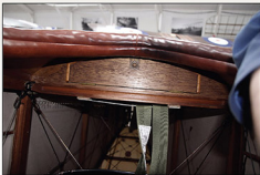
Storage locker at rear of cockpit (A12). Note the method of attaching the modern 4 point safety harness shoulder straps. The usual safety belt arrangement for RFC aircraft during WW1 was the wide 'waist belt' (P2 & P3).
