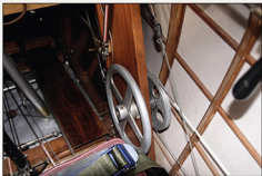
Tailplane angle of incidence adjusting wheel (B9) and pulley (B10) mounted through the right cabane strut.
