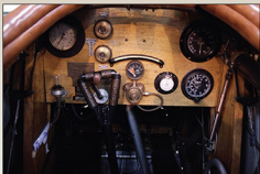
Instrument board showing one arrangement of instruments which could vary considerably from one aircraft to another. This aircraft is missing its Type 5/17 compass (B1). Note the cord wrapped around the spade grip of the control column which was not a feature of WW1 era Triplanes as far as we can ascertain.
