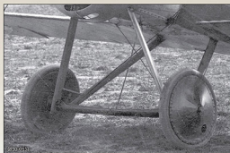
Undercarriage detail from Oakley built twin gun Sopwith Triplane N5912 seen on page 18. Note the empty shell chutes (F2) for the twin guns.
