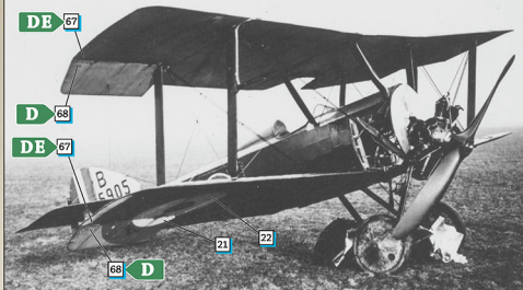
Seen here after an incident that resulted in severe engine damage, B5905 was a 100hp Gnome Monosoupape powered Sopwith Pup, from the same Standard Motor Co Ltd production order as D and E .
