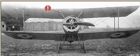
An unidentified 80hp Gnome powered Sopwith Pup. Note the non-standard slot cut in the upper face of the engine cowling.
