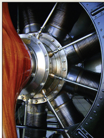
A working 100hp Gnome Monosoupe as fitted to The Vintage Aviator LTD's Avro 504. Note the castor oil staining, rocker arm and plug lead details.
