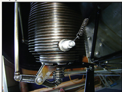
A working 100hp Gnome Monosoupe as fitted to The Vintage Aviator LTD's Avro 504. Note the castor oil staining, rocker arm and plug lead details.
