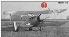
Two photos showing 100hp Gnome powered Standard Motor Co built Sopwith Pup B5903 following a forced landing. Note the lighter shade of the starboard aileron cockade.
