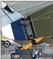
Tail skid detail of the beautiful 80hp LeRhone powered Sopwith Pup reproduction N6205 "Betty" built by The Vintage Aviator LTD.
