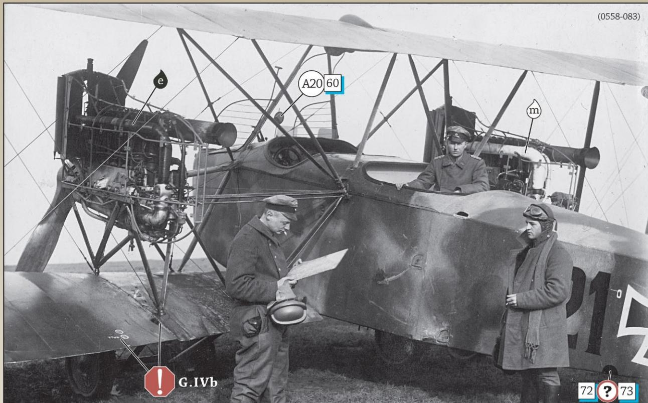
Only the additional angle of incidence markings on the bottom wing and wide gap starting near the trailing edge help identify this as an AEG G.IVb (we have not noted these details on any confirmed AEG G.IV images). Note the different coloured lagging wrapped around each carburetter intake pipe, 3 colour camouflage and the number 21 painted on the fuselage.
