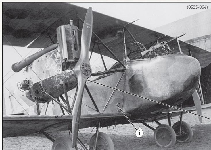
Front view of the starboard engine nacelle and nose from from captured AEG G.IV 1125/16 **D**. Note the white **i** fuel lines leading from the side of the fuselage into the bottom wing and the addition of an RFC pitot head above the cabane struts.
