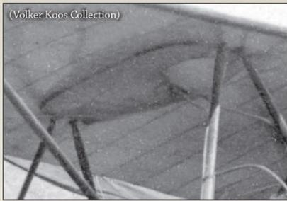
Gravity fuel tank **A14** detail from AEG G.IV 157/16 **B1**. Note the fairing over the fuel gauges **A9**.
