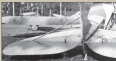
Tailplane detail from an early production Rumpler C.IV. Note the elevator control horns [D4], flat upper surface of the horizontal tailplanes and unlaced fuselage fabric.
