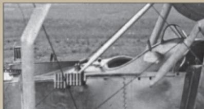
Cockpit coaming detail from crashed Rumpier C.IV 8270/16 as seen on page 13. Note the auxiliary fuel tank filler cap visible above a rack of flares  $\text{G18}$  and lever  $\text{A6}$  used to remotely cock the pilot's IMG 08 'Spandau' machine gun which appears to have an unpainted aluminium  $\text{C}$  fairing.
