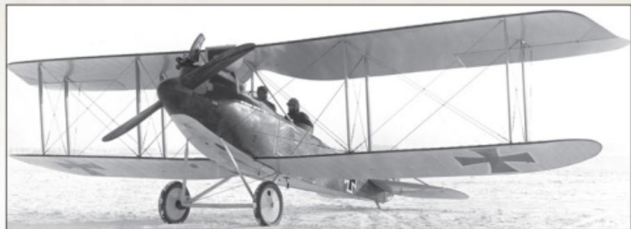
While this photo of Rumpler C.IV 8239/16 reveals many interesting details, it is important to note that some of these are unusual and not seen on normal production aircraft. These unusual details include a white surround to the port bottom wing balkenkreuz (a feature usually seen on later production aircraft), lack of wing assembly and rigging instructions [65] & [60] on the fuselage, balanced elevators and evidence of previously fitted balanced ailerons (note the modified top wing tips).
