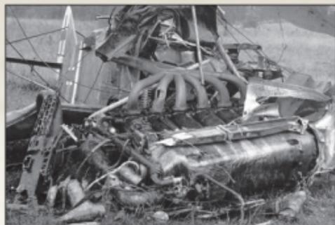
This photo of the severely damaged Rumpier C.IV 8068/17 reveals many otherwise hidden internal details such as the IMG 08 'Spandau' mount **P10** and bottom of the 260hp Daimler-Mercedes D.IV engine.
