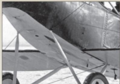
Rumpler C.IV 8239/16 displays an early style of engine air intake (H2) and full elevator control cable fairing along the centerline of the fuselage (H3). Note the wireless aerial (A47), various access hatches and the bomb doors. See page 11 for a full view of this aircraft.
