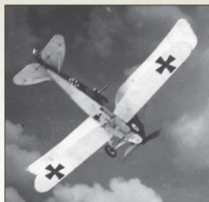
This photo of an early production Rumlper C.IV in flight allows us to see the position of the camera port, bomb sight and internal bomb rack opening on the bottom of the fuselage **113**. Also visible is the abbreviated form of fairing **118** for the elevator control cables. The wings appear brighter than the light blue tailplane and bottom of the fuselage and are probably white bleached linen **v**.
