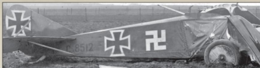
Rumpler C.IV 8512/16 showing the early fuselage with the fabric area extending under the horizontal tailplane. Despite the personal swastika marking on the fuselage it is understood that this crash occurred at a Flieger-Schule in Breig (Brzeg – Poland) during 1918 (ref. C&CJ V13#1 1972).
