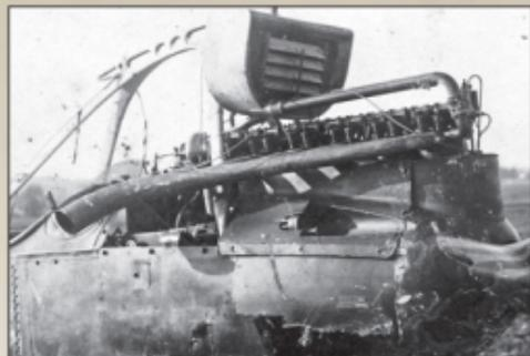
This photo of Ltms Gericke and Pfeifer's FA A 282 (Flieger-Abteilung Artillerie 282) Rumpier C.IV was taken after a crash landing and allows us to see the installation of the IMG 08 'Spandau'.
