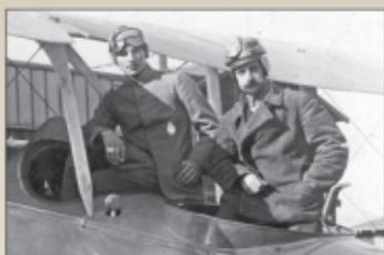
Pilot and observer cockpit coaming detail from Rumpier C.IV 6758/16  $\text{B}$  showing windshield  $\text{C1}$ , Maximal fuel gauge  $\text{A43}$  +  $\text{90}$  and standard Parabellum mount  $\text{G4}$  +  $\text{G9}$ .
