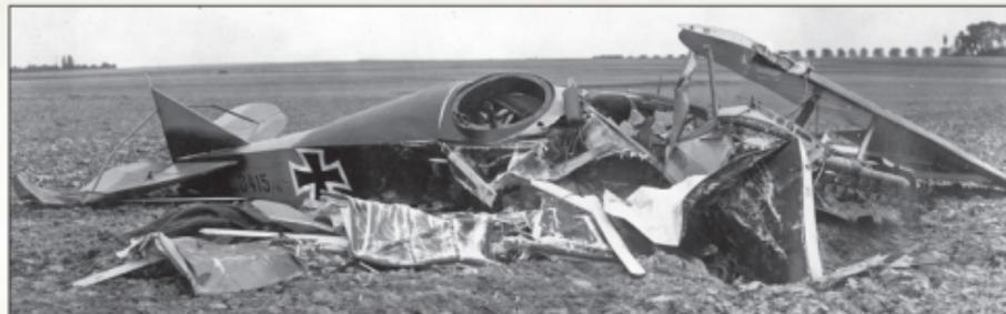
The sad wreckage of Rumpler C.IV 8415/16 allows us to see many otherwise hidden details. Note the light blue metal tubes of the fuselage structure visible in the observer's cockpit, cabane struts (84) & (89) and what appears to be additional seat back padding for the pilot. 8415/16 was from the 3rd production batch of 150 aircraft ordered in November 1916 and was destroyed before its fuselage could be reinforced.
