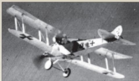
This unidentified Rumpler C.IV has an abbreviated form of elevator control cable fairing (H3). Note the bomb doors, open camera port and rounded nose (A25). Unfortunately the fuselage Wappen (heraldic shield) marking is not legible.
