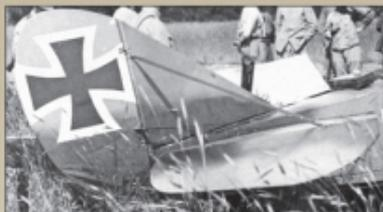
Fin and rudder detail from captured Rumpler C.IV showing the rudder eisenkreuz [6] & [5]. The box visible on top of the fuselage is a first aid kit [G5] + [G15].
