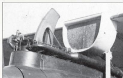
Windhoff radiator **B11** + **B12** from 6758/16 **B**. Note the short exhaust **A57** and support bracket **A58**.
