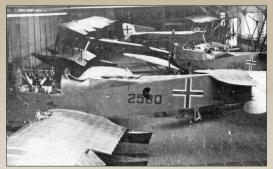
C2MGHFT W.29s 2580 and 2583 await demolition at Wilhelmshaven after the armistice. Both aircraft were from a batch of 20 C2MGHFT W.29s (numbers 2564 to 2583) ordered in late May 1918 and feature late production tailplanes (B9). The neter has been removed from 2580 and neither aircraft has any weapons fitted. What appears to be a hole in the side of 2580 is damage to the photograph negative.
