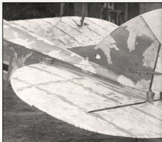
Note the control horn and cable outlet details on the tail of 1562/18 w/n (work number) 4012.
