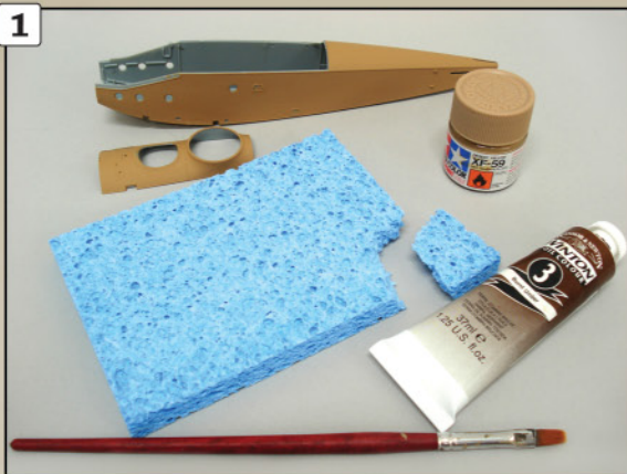
Equipment needed shown - Base coat area using XF59.
