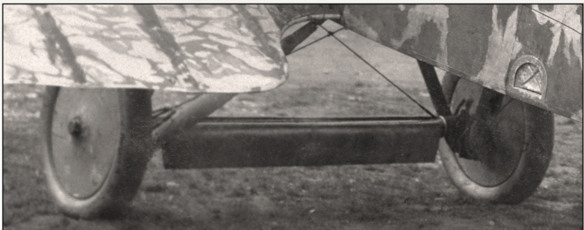
Undercarriage detail from LVG C.VI 1562/18 w/n 4012 showing the axle wing hanging down.
