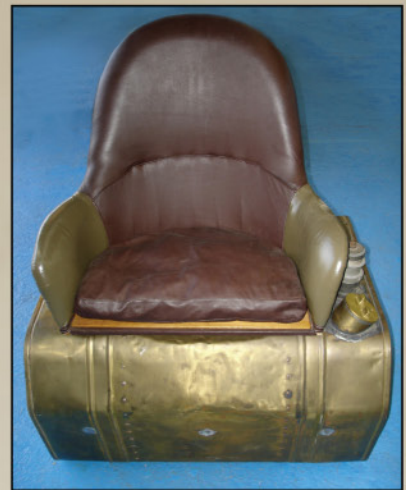
Seat and fuel tank detail from LVG C.VI 9041/18 undergoing restoration at the Memorial Flight Association at the Musée de L'Air. Note the unpainted brass fuel tank (Memorial Flight Association).
