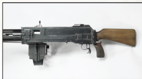
15 The observers main defensive weapon was the Parabellum LMG14 (shown here) or the later LMG14/17. The 200 round drum magazine has been removed for the photo.
