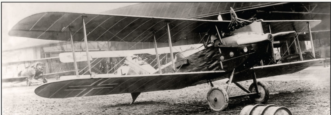
A nice post armistice view showing the light coloured clear doped linen rib tapes and engine 'winter cowl' fitted. Additionally we can see another style of flare or grenade rack and the deformed plywood fuselage sides (via Colin Owers).
