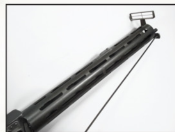
15 The observers main defensive weapon was the Parabellum LMG14 (shown here) or the later LMG14/17. The 200 round drum magazine has been removed for the photo.
