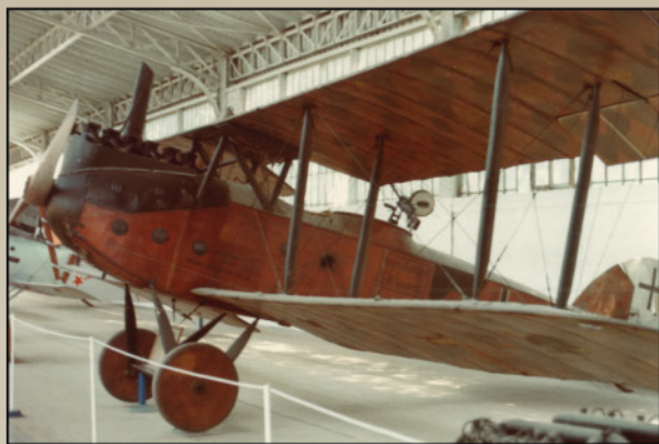
LVG C.VI 4981/18 appearing remarkably original when pictured here in the Brussels Air Museum. Of note is the lightly stained fuselage, dark engine panels, unusual exhaust and wooden wheels.
