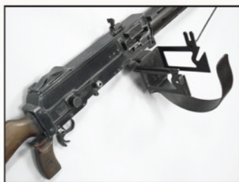
15 The observers main defensive weapon was the Parabellum LMG14 (shown here) or the later LMG14/17. The 200 round drum magazine has been removed for the photo.
