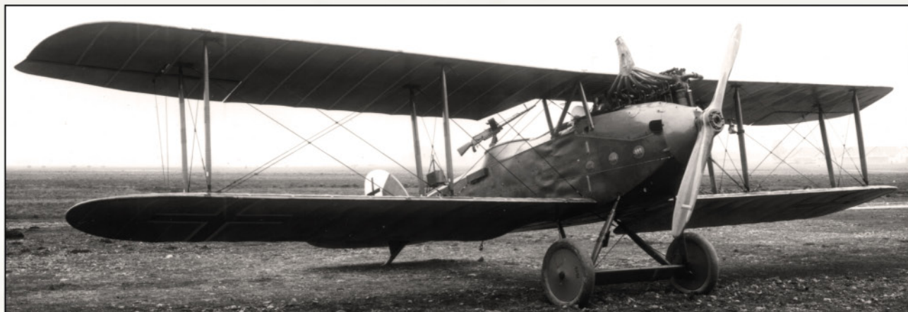
LVG C.VI w/n 4821. Note the Barograph strung between the inner starboard struts and deformed plywood fuselage (via Colin Owers).
