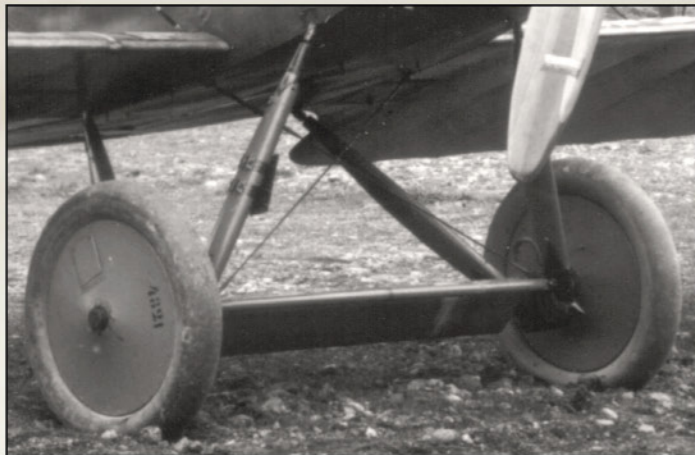
Undercarriage detail from LVG C.VI w/n 4821 (via Colin Owers).
