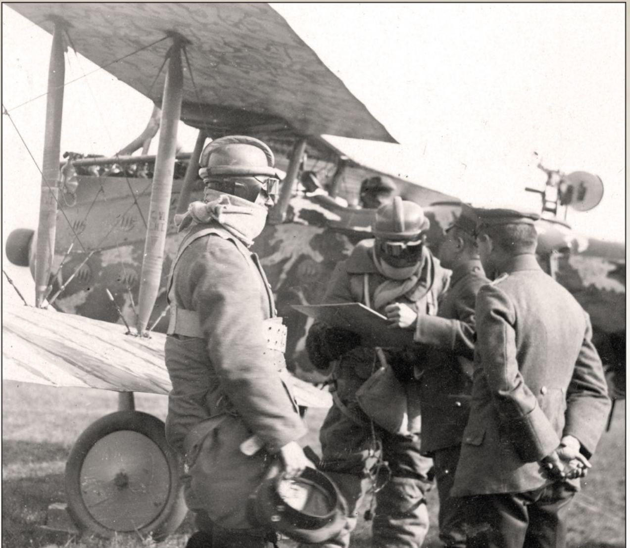
A ground crewman warms up LVG C.VI 1562 w/n 4012 while Lt Kuchenthal and Uffz Friedmeyer get their last minute pre-flight briefing. Note the application of camouflage paint on the lower surface of the upper wing.
