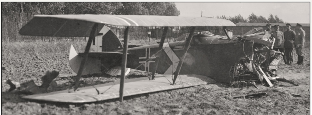
9 The crash landing of Oblt Konsek's LVG C.VI, possibly 4821/18, proves of interest to a group of onlookers. The uneven arms on the fuselage Balkenkreuz date this photo to sometime after the middle of May 1918.
