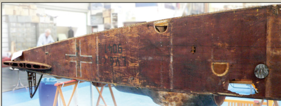
LVG C.VI 9041/18 undergoing restoration at the Memorial Flight Association. The original condition of the fuselage allows us to see the dark red brown stain applied to the exterior (Memorial Flight Association).
