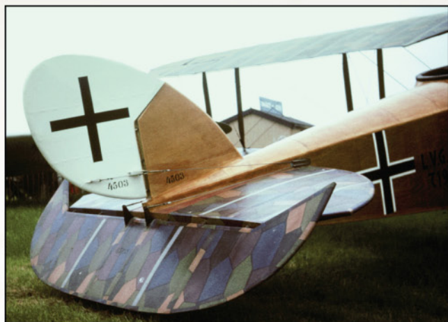
Tailplane detail from Shuttleworth's LVG C.VI 7198/18 w/n 4503. Note the unusual strips of lozenge material on the elevator (Ray Rimell).
