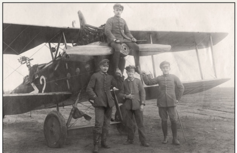
LVG C.VI '2' displaying yet another flare rack arrangement. Note the instrument, possibly a rate of climb indicator, suspended from the rigging in front of the cockpit.
