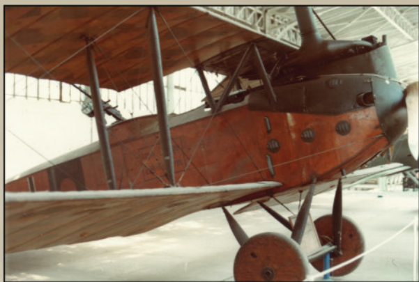
LVG C.VI 4981/18 appearing remarkably original when pictured here in the Brussels Air Museum. Of note is the lightly stained fuselage, dark engine panels, unusual exhaust and wooden wheels.
