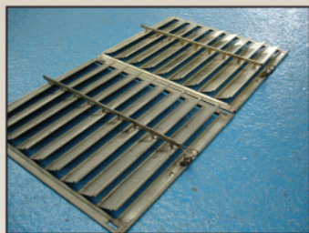
Restored and reproduction adjustable radiator shutters. These were operated by the handle shown in the above photo of 1562/18 (Memorial Flight Association).
