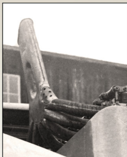
Another style of exhaust as seen on this LVG C.VI, possibly w/n 4008.
