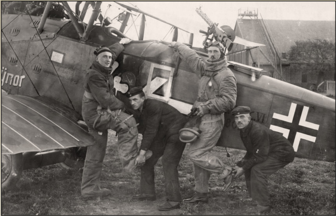
LVG C.VI 4802/18 "Eleanor" with Lt Weymar and Lt Haselhoff getting a helping hand before their mission on 18 September 1918. Of interest is the added sliding lid over the compartment to the rear of the observer's cockpit and the 'rack' on the side of the fuselage. Also note the dark tape running along the edges of the fuselage.
