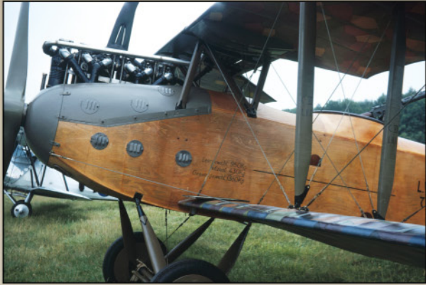
Nose detail from the Shuttleworth Collection's LVG C.VI 7198/18 showing the strut end brackets, turnbuckles and rigging details. Also note the very dark engine cowlings and light varnished fuselage (Ray Rimell).
