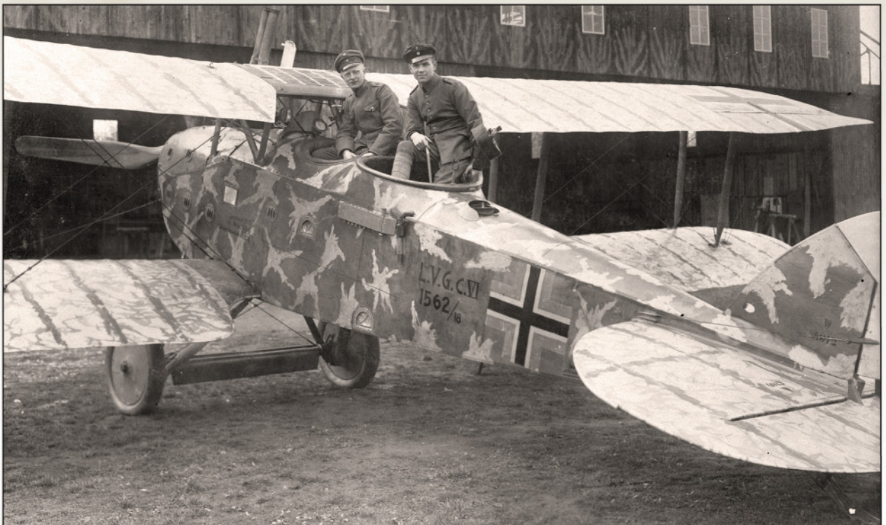
LVG C.VI 1562 w/n 4012 with Lt Kuchenthal and Uffz Friedemeye. Note the interesting winter camouflage application, externally mounted compass, flare gun and modified, thinner, Balkenkreuz marking dating this photo to some time after the middle of May 1918.
