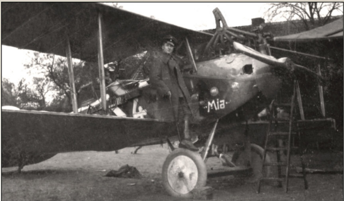
Lt Weymar striking a pose on the other side of LVG C.VI 4802/18 displaying the name 'Mia', possibly the name of a loved one. Of note here is the vast array of racks amassed below the observer's cockpit and a generator dynamo attached to the starboard undercarriage leg.
