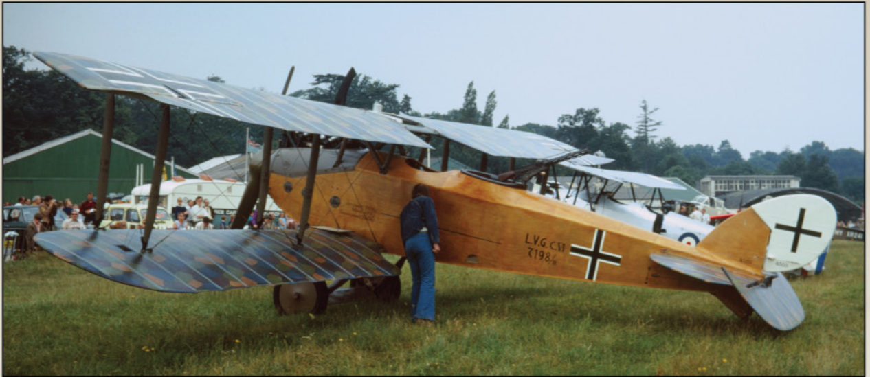
The Shuttleworth Collection's beautifully restored aircraft. Note the aileron washout, non-standard blue rib tapes and the flared trousers on the aviation enthusiast inspecting the fuselage wood grain, dating this photo to sometime after 1969 (Ray Rimell).
