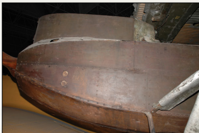
Original red oxide primer under camouflage colours (586/18 Canada).
