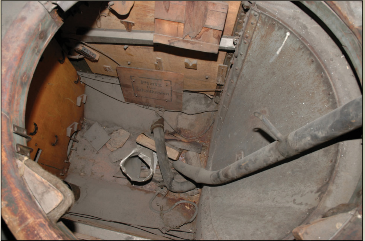
Rear observer/gunner cockpit. Unfortunately many fittings are missing. Note 'horseshoe' mounts on bulkhead for the radio (586/18 Canada).
