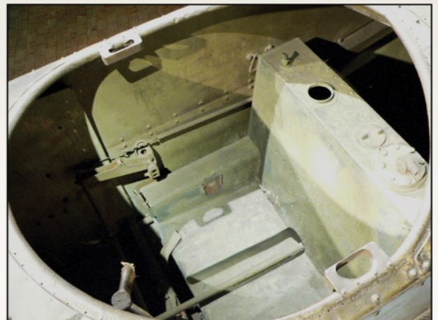
The stripped fuel tank which makes up most of the pilot's seat (Berlin).
