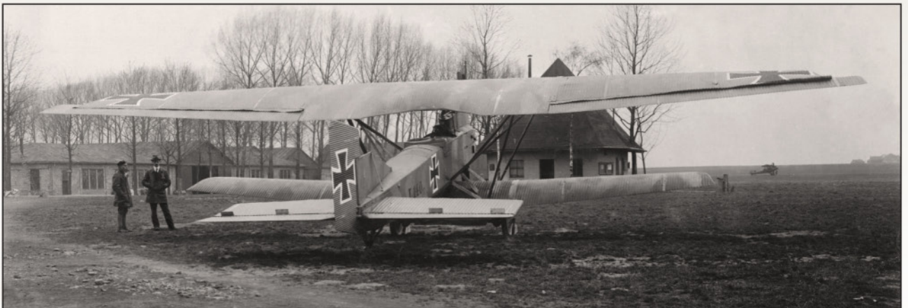
Another view of 140/17 showing the Junkers J.1 thick wing profile.
