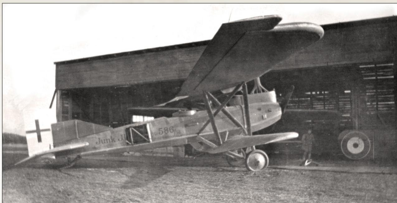
Note the 5 colour lozenge camouflage fabric on the rear fuselage of 586/18. This aircraft is now located in the Canada Aviation Museum.
