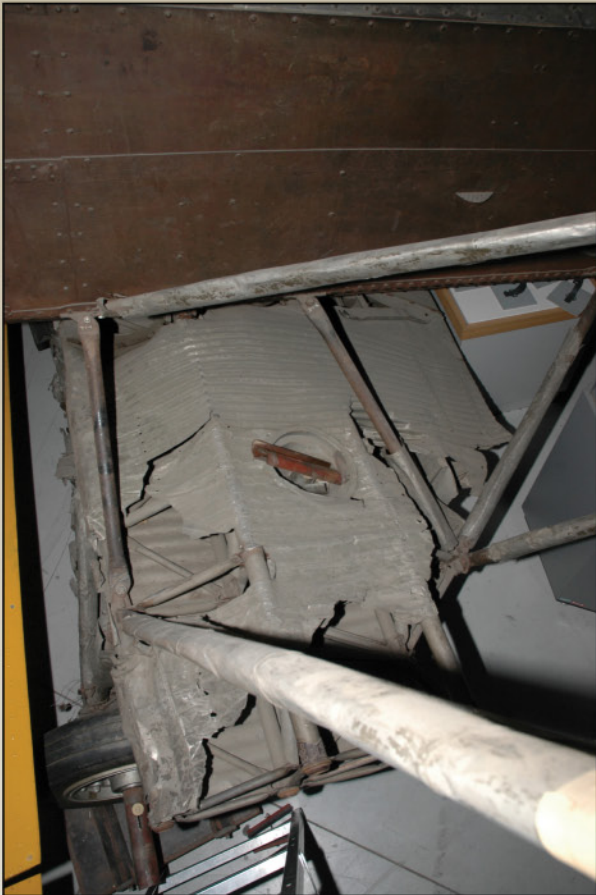
Hole in lower left wing for compass (586/18 Canada).
