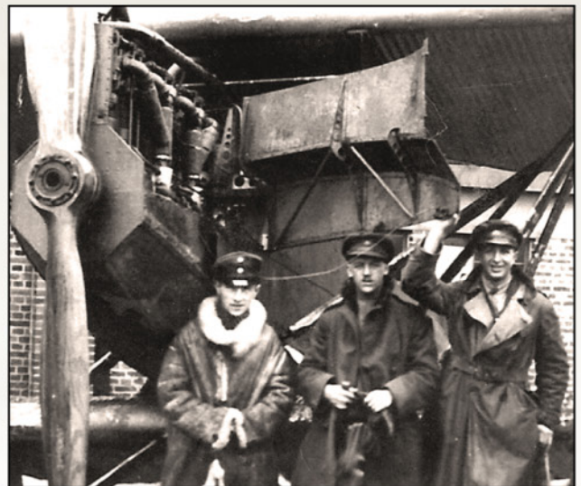
Note engine bay interior bracing of this captured Junkers J.1.
