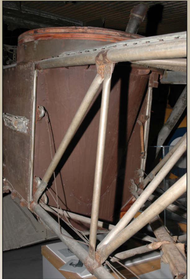
Elevator and rudder control cables exiting the rear of the armoured fuselage section (586/18 Canada).
