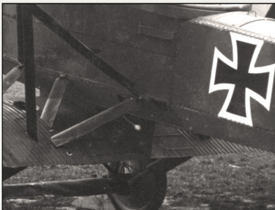
Note the compass and radio aerial details in this close up of 140/17.
