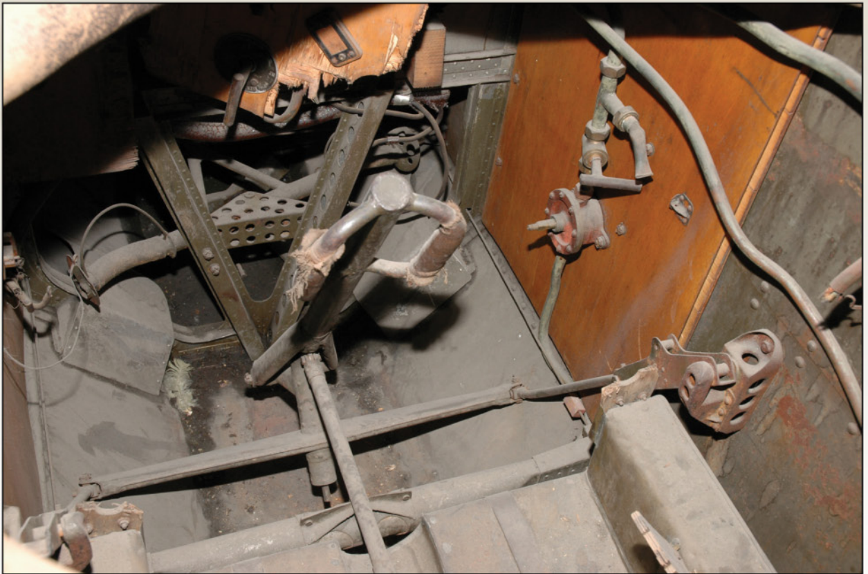
Pilot's cockpit of 586/18. Note the unusual aileron crank arrangement.
