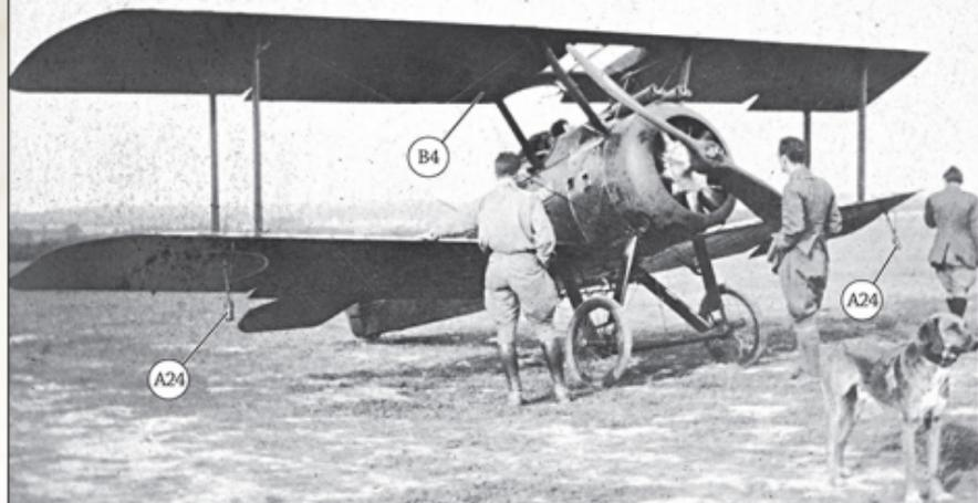
110hp Le Rhône 9J powered Sopwith F.1 Camel C6713 'Doris' was from an production order for 100 aircraft placed with the British Caudron Co Ltd in August 1917 and was equipped for night flying duties with 78 (HD) Sqn in January 1918. It is seen here after it was serving in 151 Sqn in mid 1918. Note the Holt flares, bomb carrier, subdued bottom wing cockade and large centre section cutout. The uncovered wire wheels are very rarely seen on operational aircraft.
