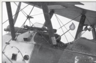
^ Cockpit decking detail from the 110hp Le Rhône 9J powered 54 Sqn Sopwith E.1 Camel B5243 "20" of WG Ivamy which was captured on 18 March 1918. Note the cut down starboard decking, Rotherham petrol pump, windscreen and Aldis sight. Difficulty in clearing starboard gun stoppages lead to many aircraft having the cockpit decking cut away in the area.
