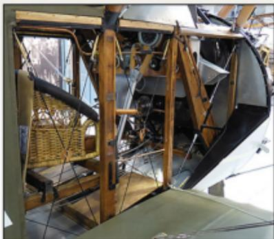
Interior fuselage detail from Sopwith F.1 Camel B5663 nearing completion of its restoration to flying status at The Vintage Aviator Ltd (TVAL) in late 2014. The front engine plate, bent & rear undercowls, magazines and carburettor induction pipes are bare aluminium while most metal brackets and fittings are painted black except for the petrol lines, sight gauge and engine control levers which remain copper and brass.
