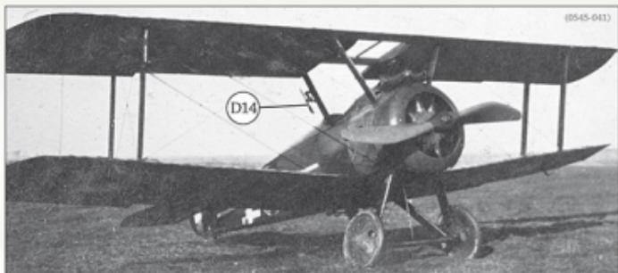
An unidentified 110hp Le Rhône 9J powered 46 Sqn Sopwith F.1 Camel, either "E", "Z" or "Z". Note the Cooper bomb carrier under the fuselage and large centre section cut out.
